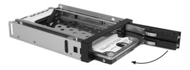
Repeat this procedure to install a second 2.5" SATA drive, into the remaining bay:
